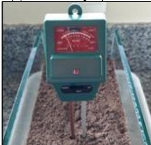
Figure 3 – Equipment for measuring temperature, humidity and pH
