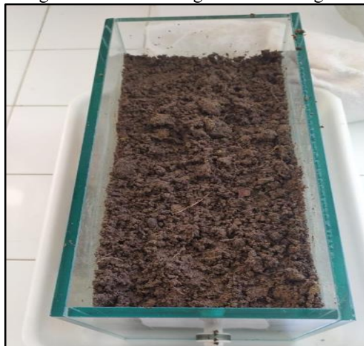
Figure 2 - Landfarming bioreactor in glass
