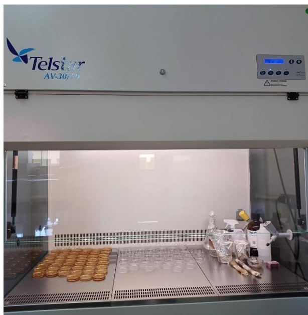
Figure 1 – Aseptic laminar flow chamber, where the inoculation of the sampled peanut grains in culture medium was performed.
